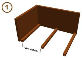
Place the joist on the ground Joist Span: 450MM
