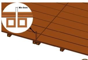
Make sure that the gap between the end of decking should be at least 6mm.
